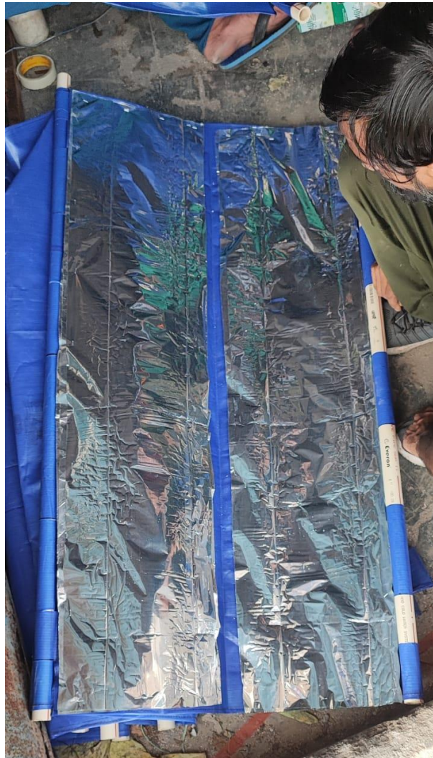
Figure 7.11: Attaching MLP to Tarpaulin
