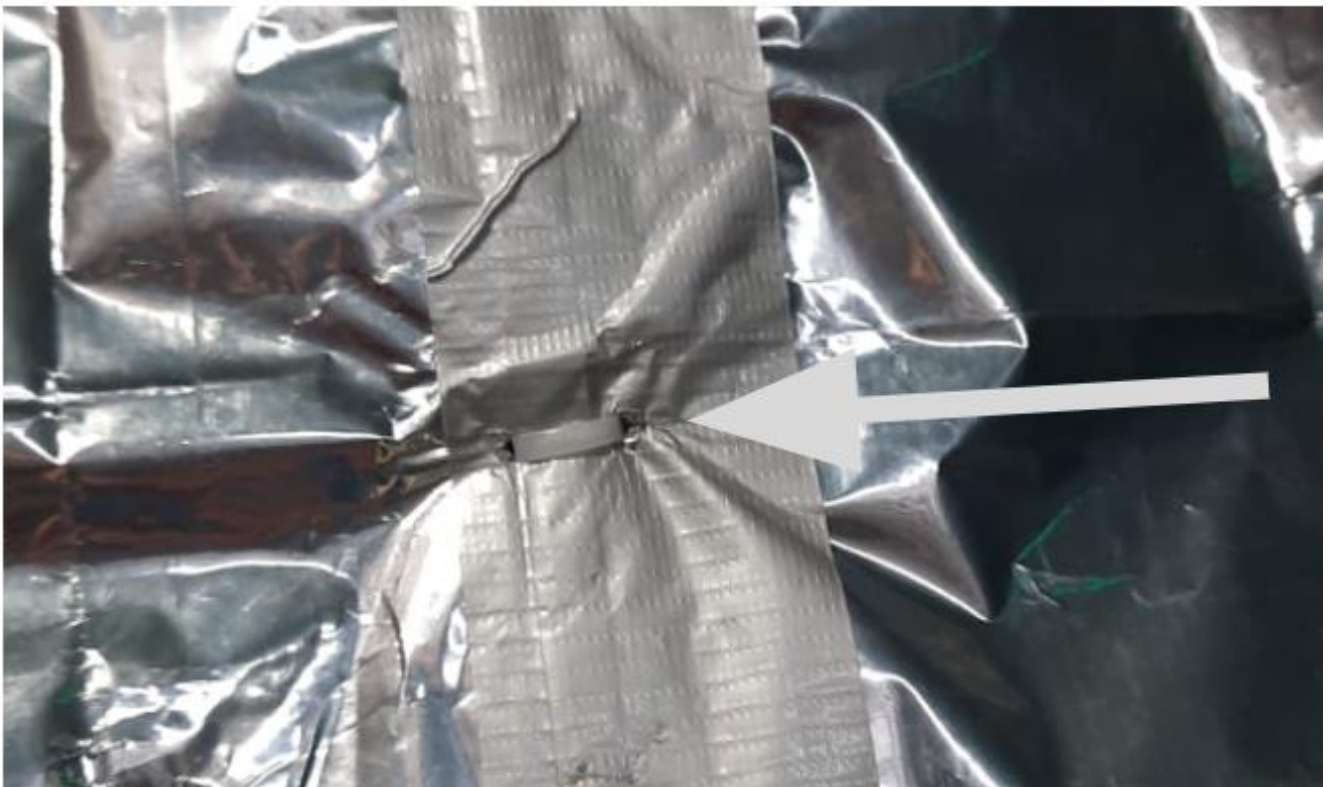
Figure 1.8: Attaching MLP and Astar fabric together with ziplock using Ductape
