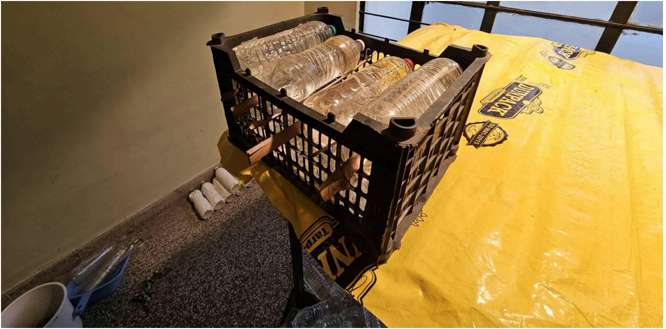
Figure 3.8 Bamboo Sticks For Adequate Spacing Between First And Second Layer(Top View)
