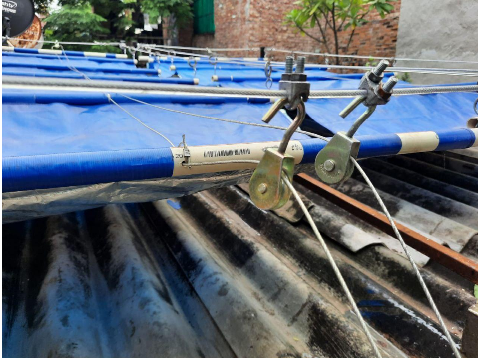
Figure 7.18: Placement of pulleys on front and rear end of the fractal along with handling mechanism
