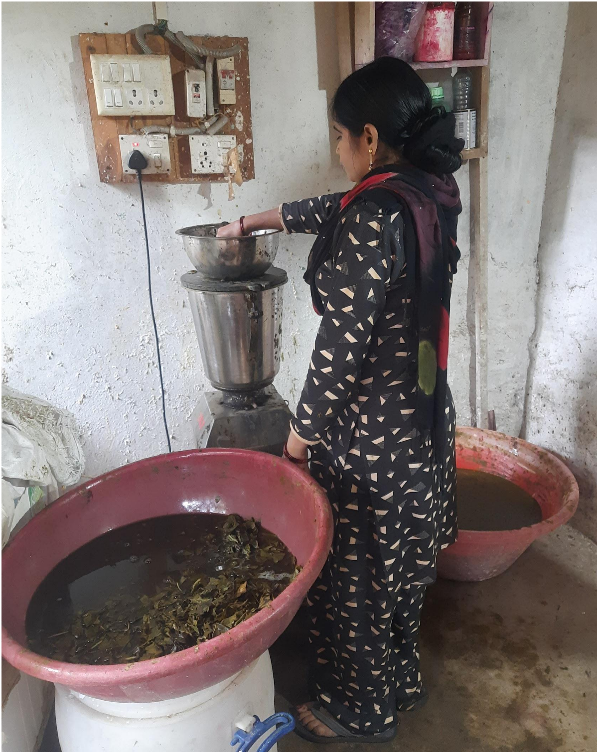
Figure 2.9: Grind the boiled fibres to a pulp in an industrial mixer
