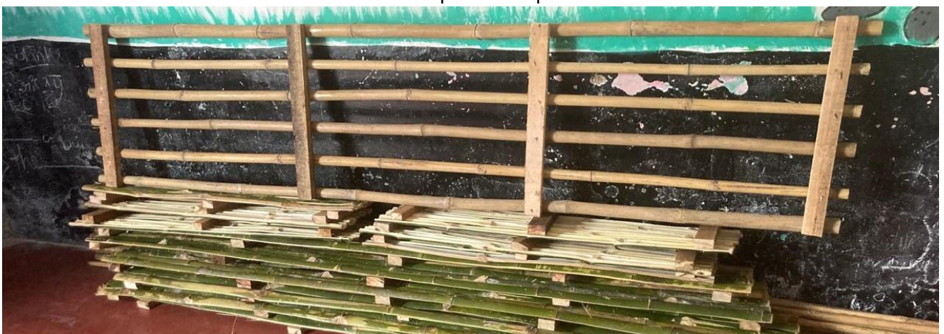
Figure 4.4: Bamboo Frame After Fabrication
