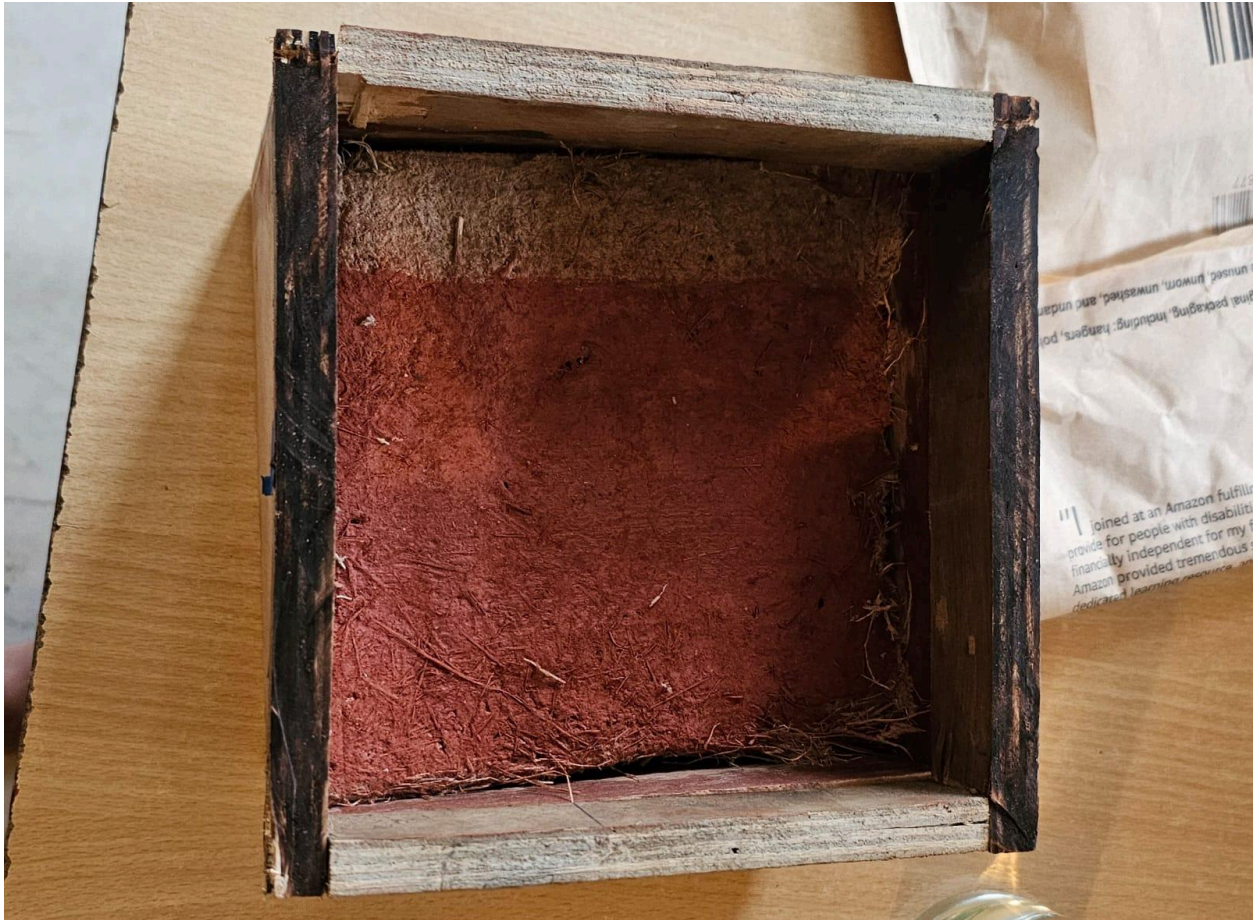
Figure 8.2 Biomass Panel Testbed (Top View Without GI Sheet)
