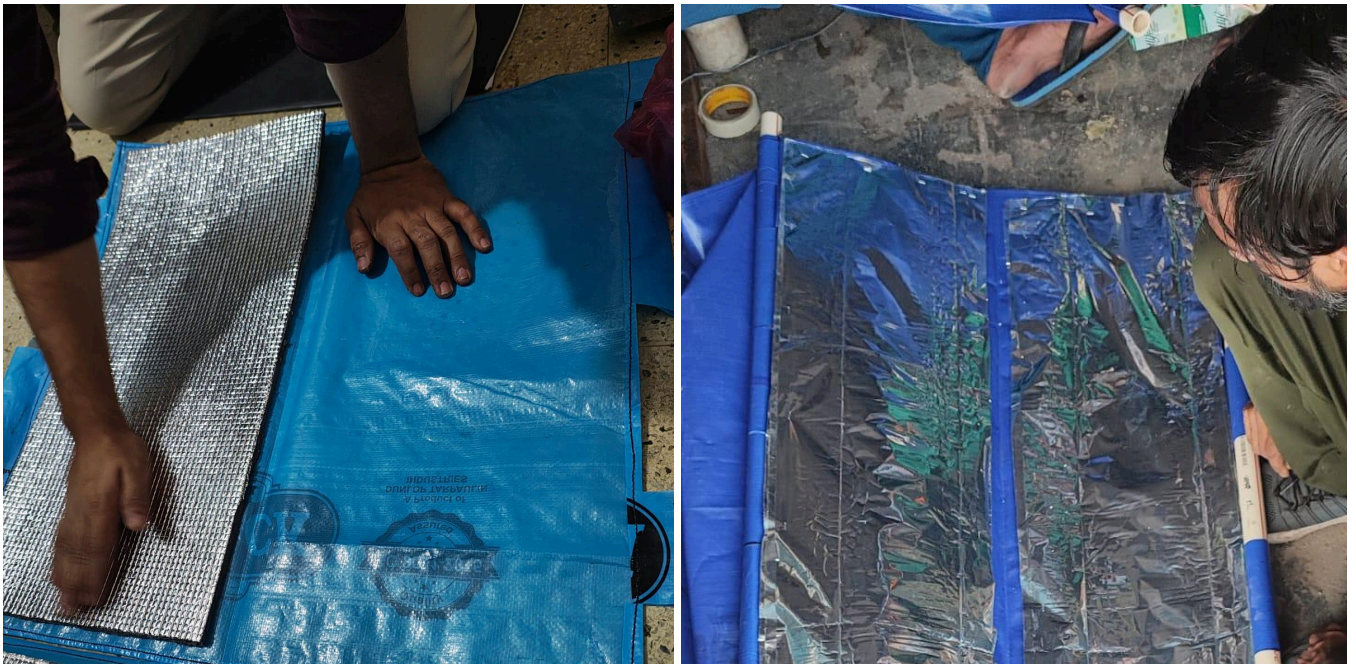
Figure 4.3 Prototype 1 With Alufoil(An Industrial Product) As Low Emissivity Barrier And Prototype 2 On The Right With Mlp Sheets For The Same Function(Made Inhouse)
