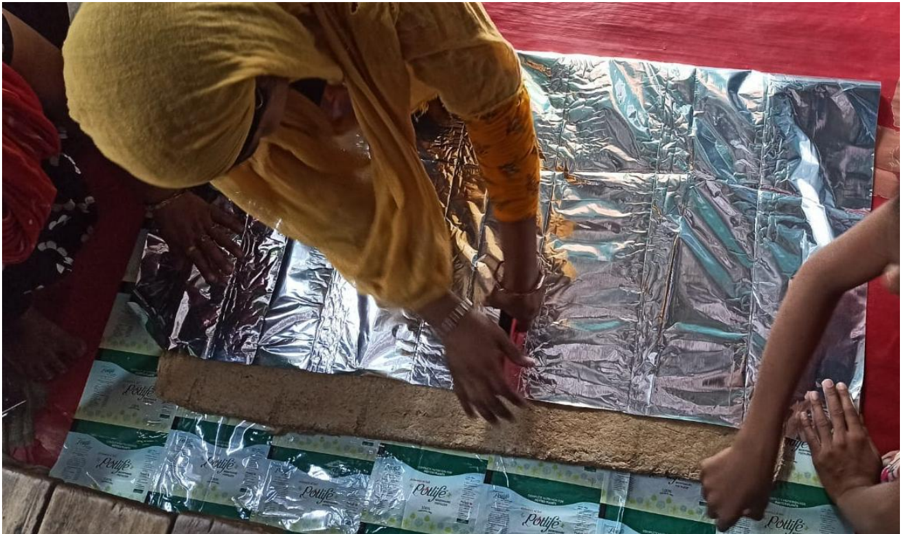
Figure 2.14: Wrap the panel with shiny surface facing outside and staple it
