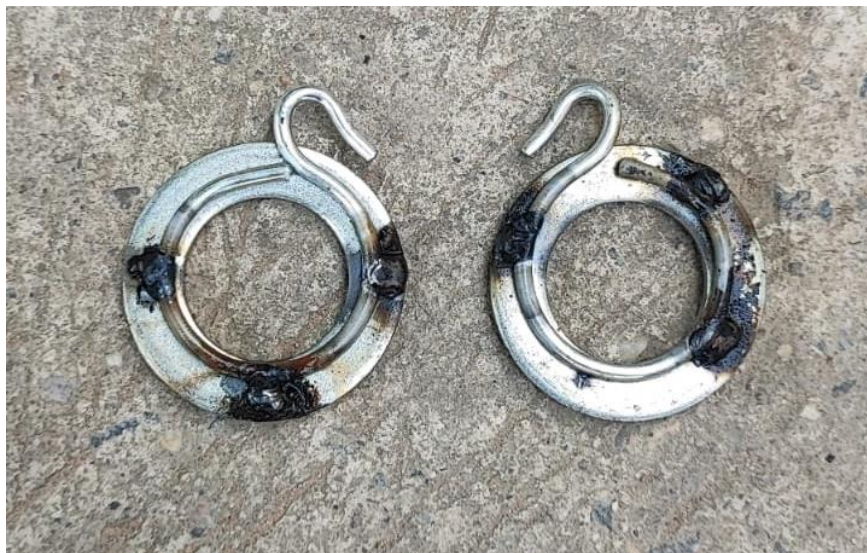
Figure 7.15: Welding washer to metal curtain rings
