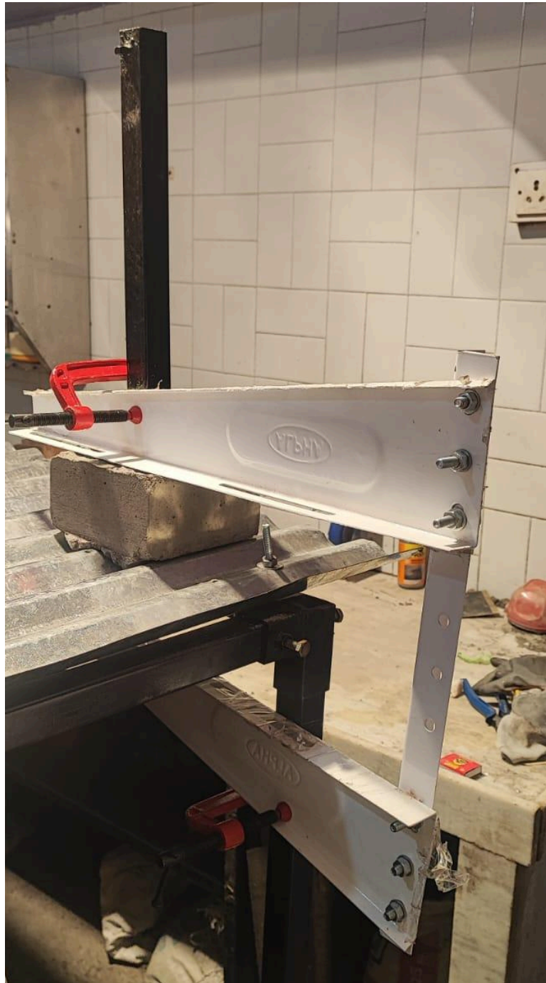
Figure 4.2 Prototyping The Clamp-Based Support For Space Frame
