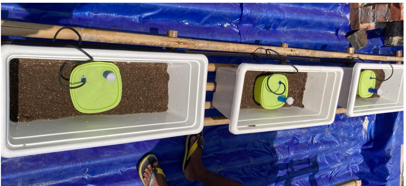
Figure 4.9: Float Valve Box Attached with Irrigation Hose and Pot
