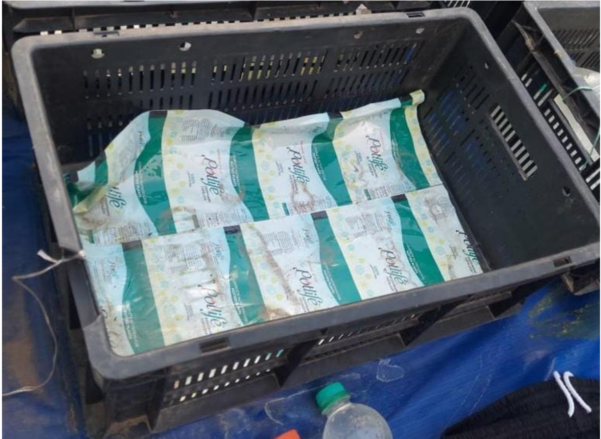
Figure 6.6: Placing Of MLP Sheets Inside The Crate
