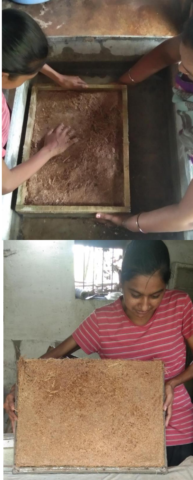
Figure 2.10: Lay out the fibres in a wooden mould within a water tank
