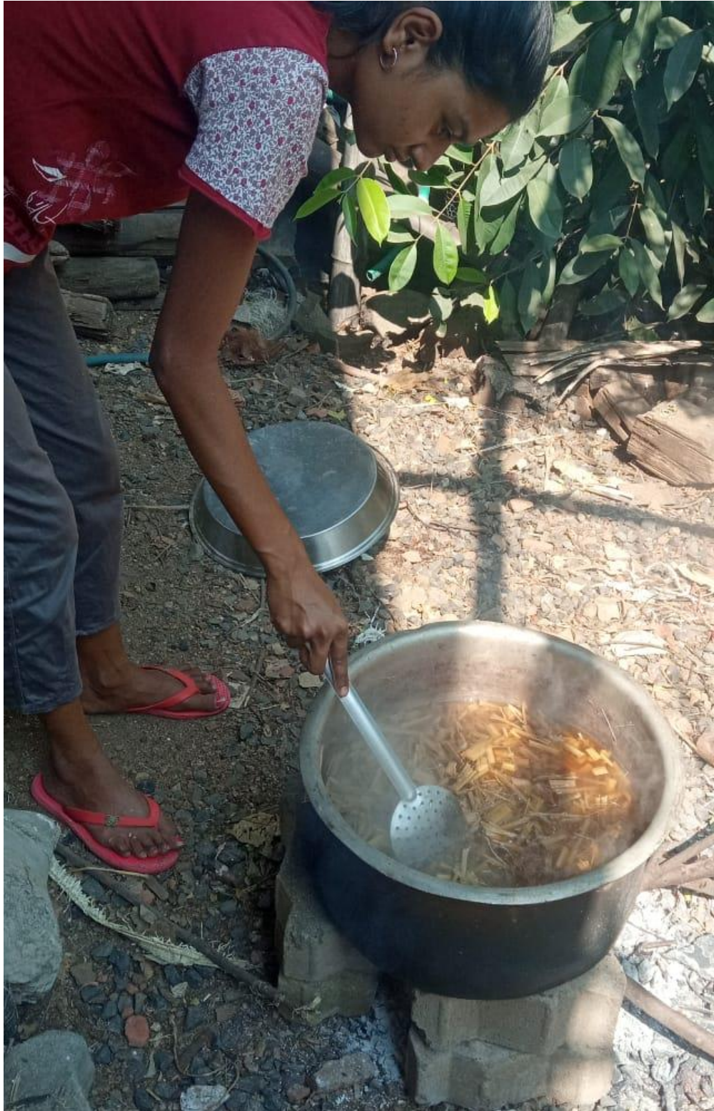
Figure 2.8: Boil the fibre pieces in sodium carbonate (soda ash)
