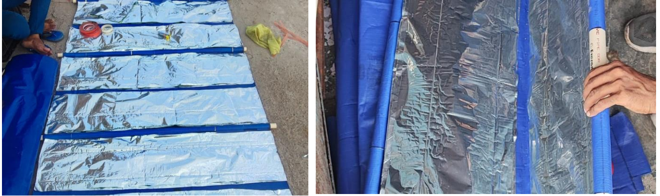
Figure 7.14: Inserting intermediary PVC pipes to make the fractal.
