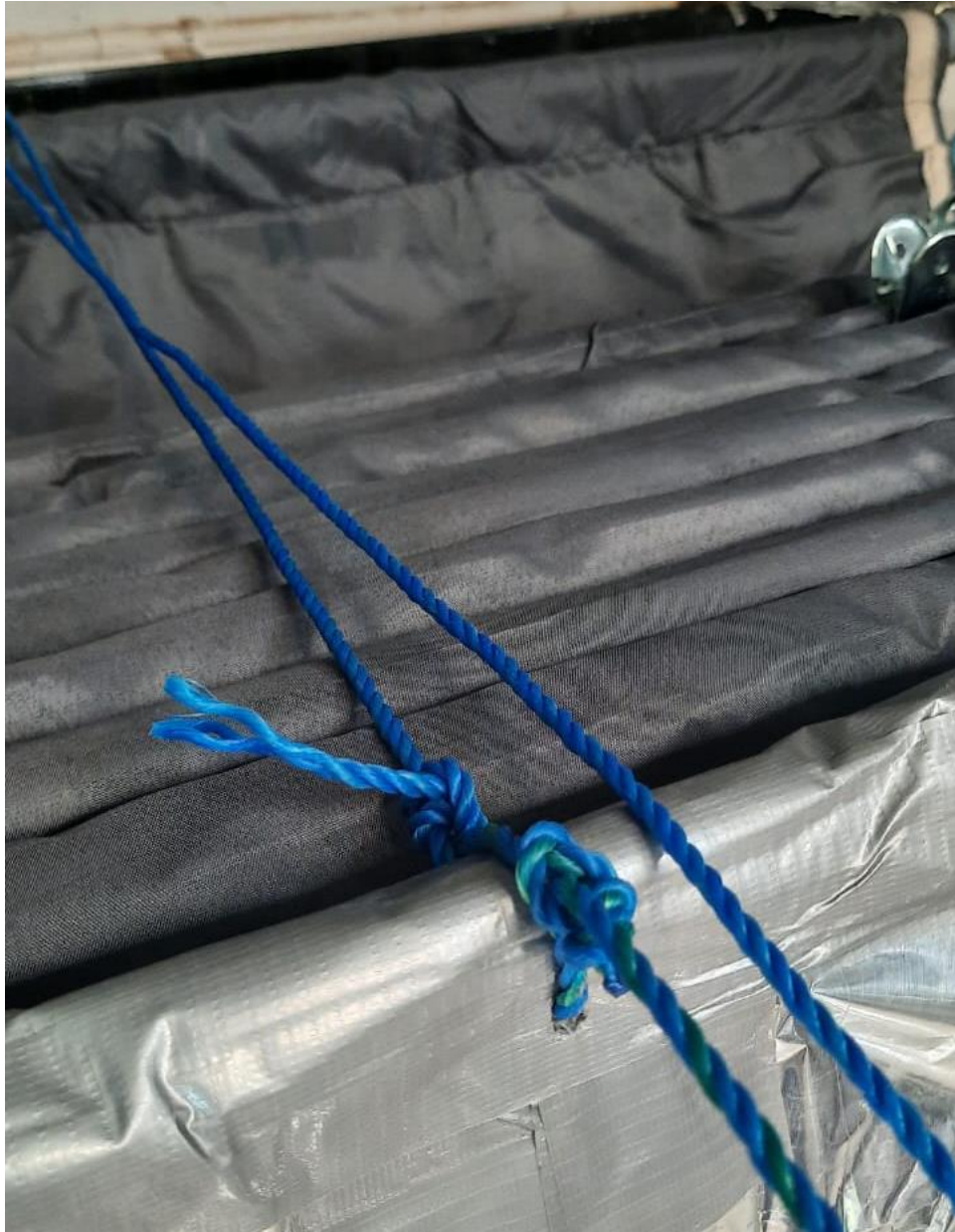
Figure 1.13: Attaching nylon rope to the front end pipe of the fractal
