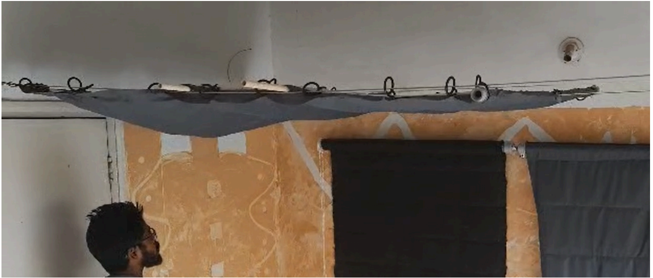
Figure 6.2 Prototype 2 With Intermediary Supports
