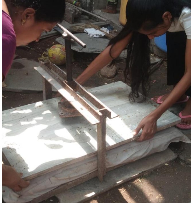
Figure 2.1: Press the panels to remove excess water
