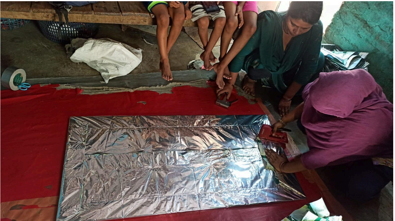
Figure 9.3 Wrapping Wood Wool Panel With MLP
