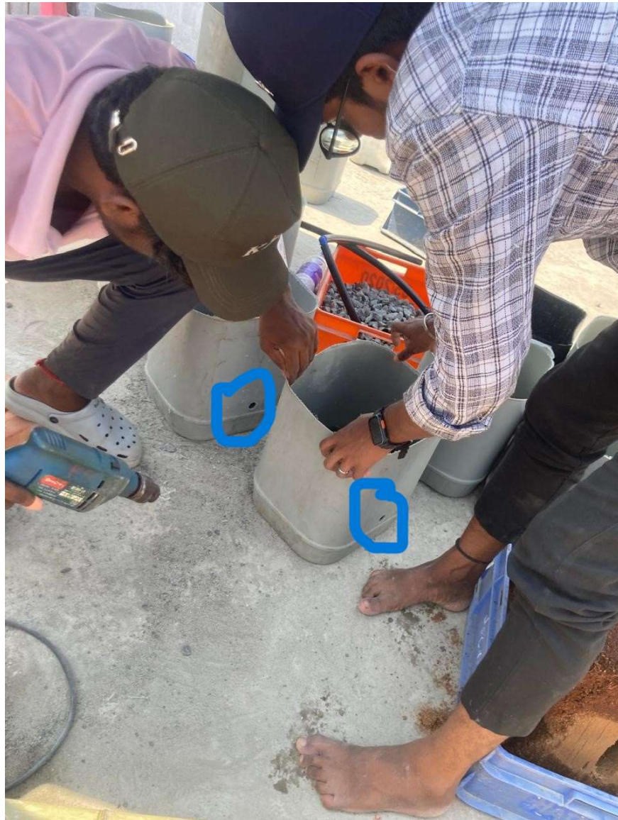
Fig 37.4.2-3 : Making 20mm hole with driller
