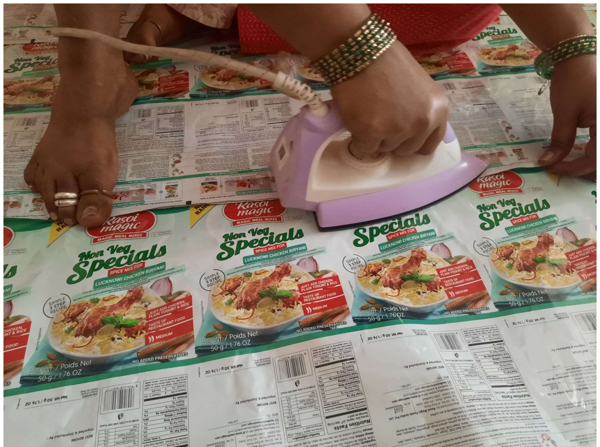
Fig 37.1.2-9 : MLP Sticking using Iron
