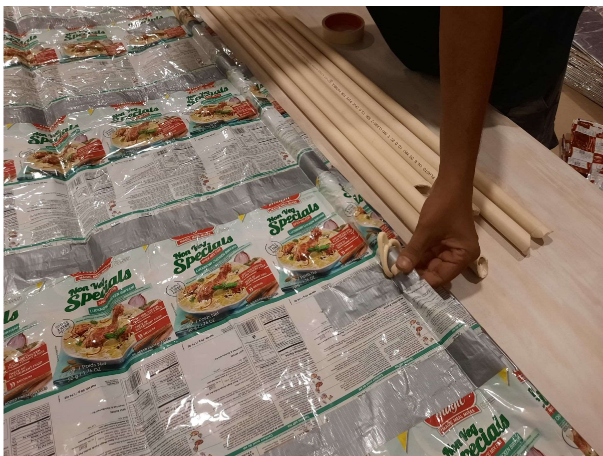
Fig 37.1.2-19 : Placing curtain hooks into the slit, inserting the UPVC pipe through the MLP loop, and passing it through the curtain hook to lock it in place.
