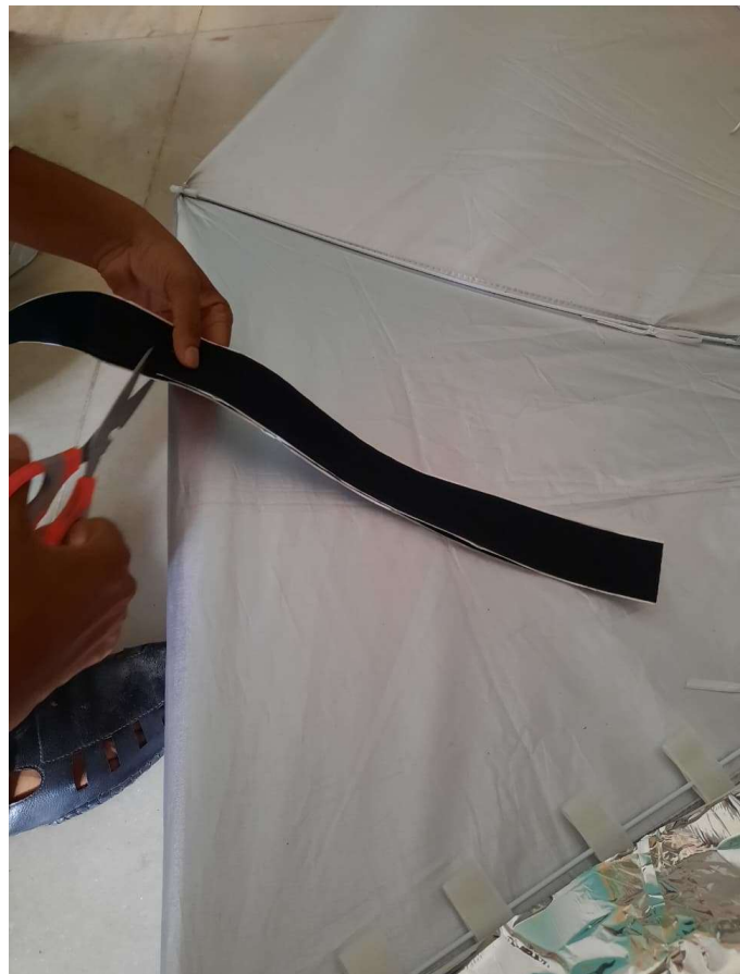
Fig 37.9.2.1.1-1 : Measuring & Cutting the velcro strip to the exact length of the spoke
