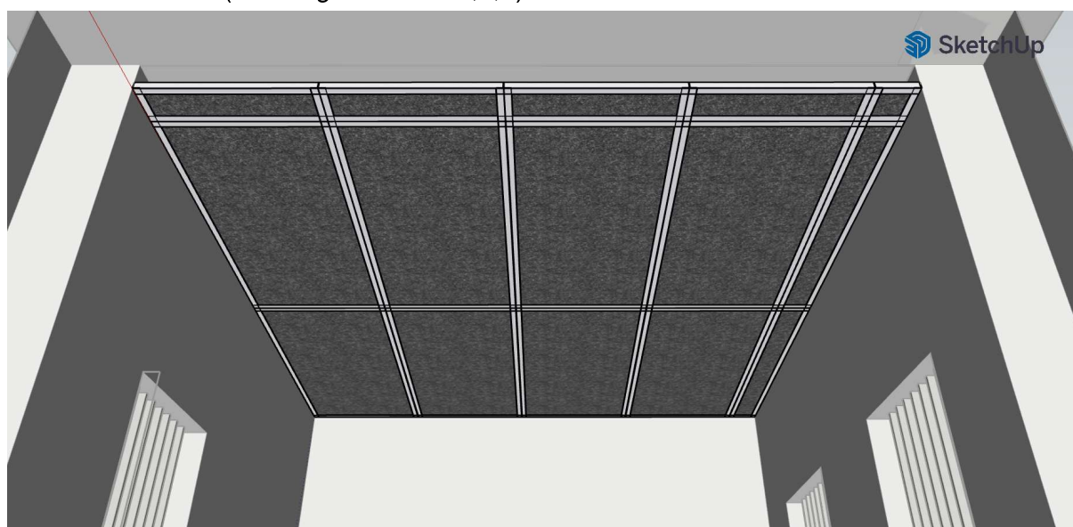
Fig 37.3.2-4 : Metal support framework with panels in place
