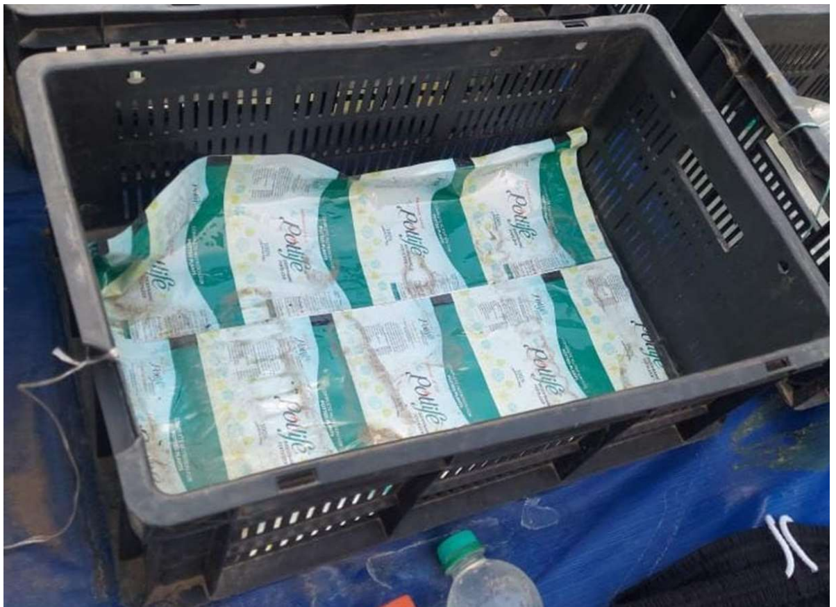
Fig 37.6.3-4 : Placing Of MLP Sheets Inside The Crate
