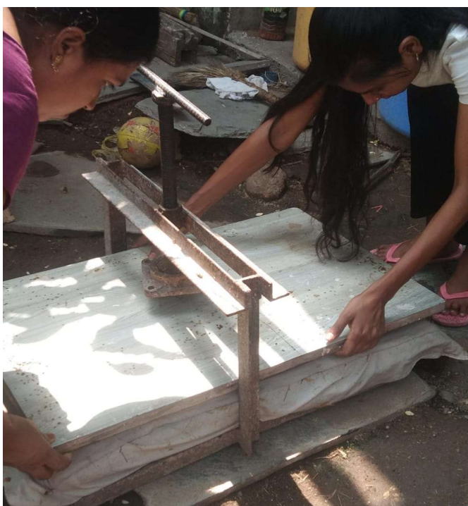
Fig 37.2.2-11: Press the panels to remove excess water
