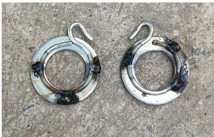
Fig 37.7.2-17 : Welding washer to metal curtain rings
