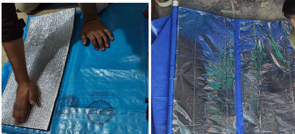
Fig 35.2.2-1 : Left image: Prototype 1 with Alufoil (an Industrial Product) as Low Emissivity Barrier Right Image: Prototype 2 with MLP Sheets for the Same Function (Made Inhouse)
