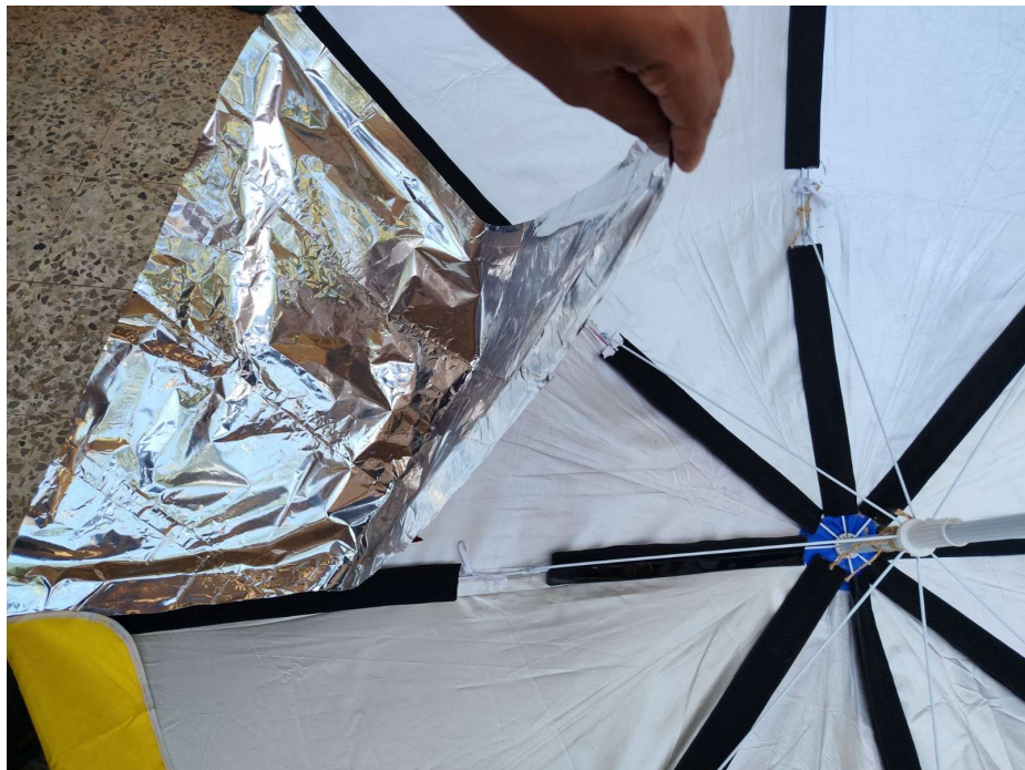
Fig 35.8.1-11 : MLP sheets Bonded Together
