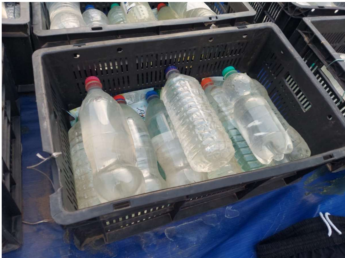
Fig 37.6.3-5 : Placement Of Bottles In Crates (Second Layer Sits In The Gap Of First Layer)
