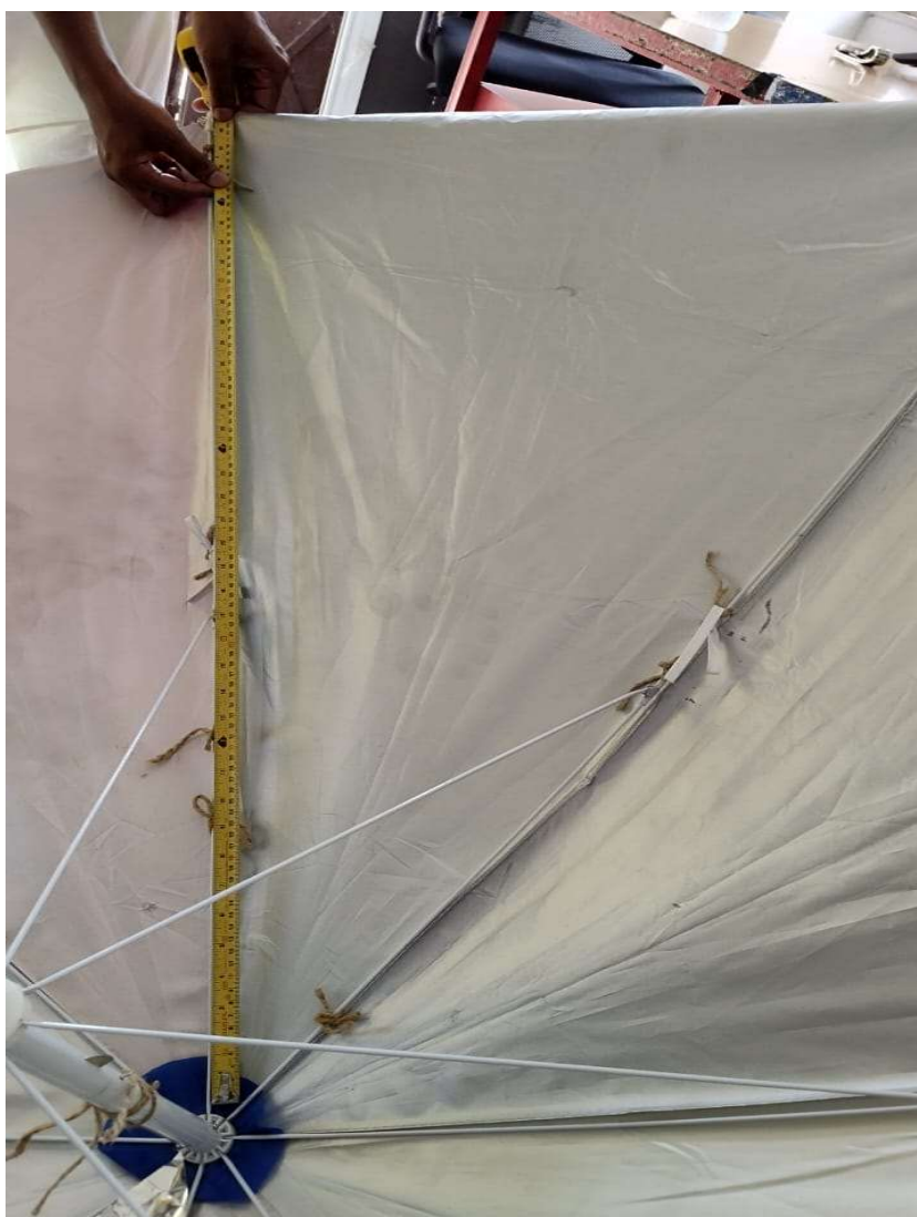
Fig 37.9.2-1 : Measuring the underside of the Umbrella spoke length and segment dimensions
