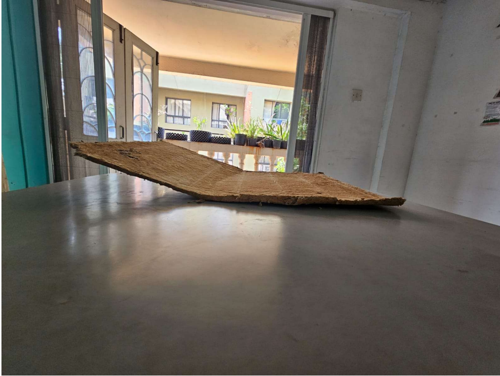
Fig 37.2.3-4 : Check for warping/bending
