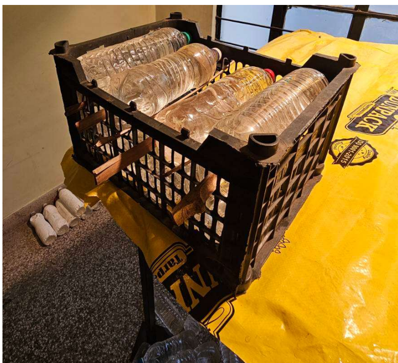
Fig 35.1.1-7 : Bamboo Sticks for Adequate Spacing Between First and Second Layer (Top View)
