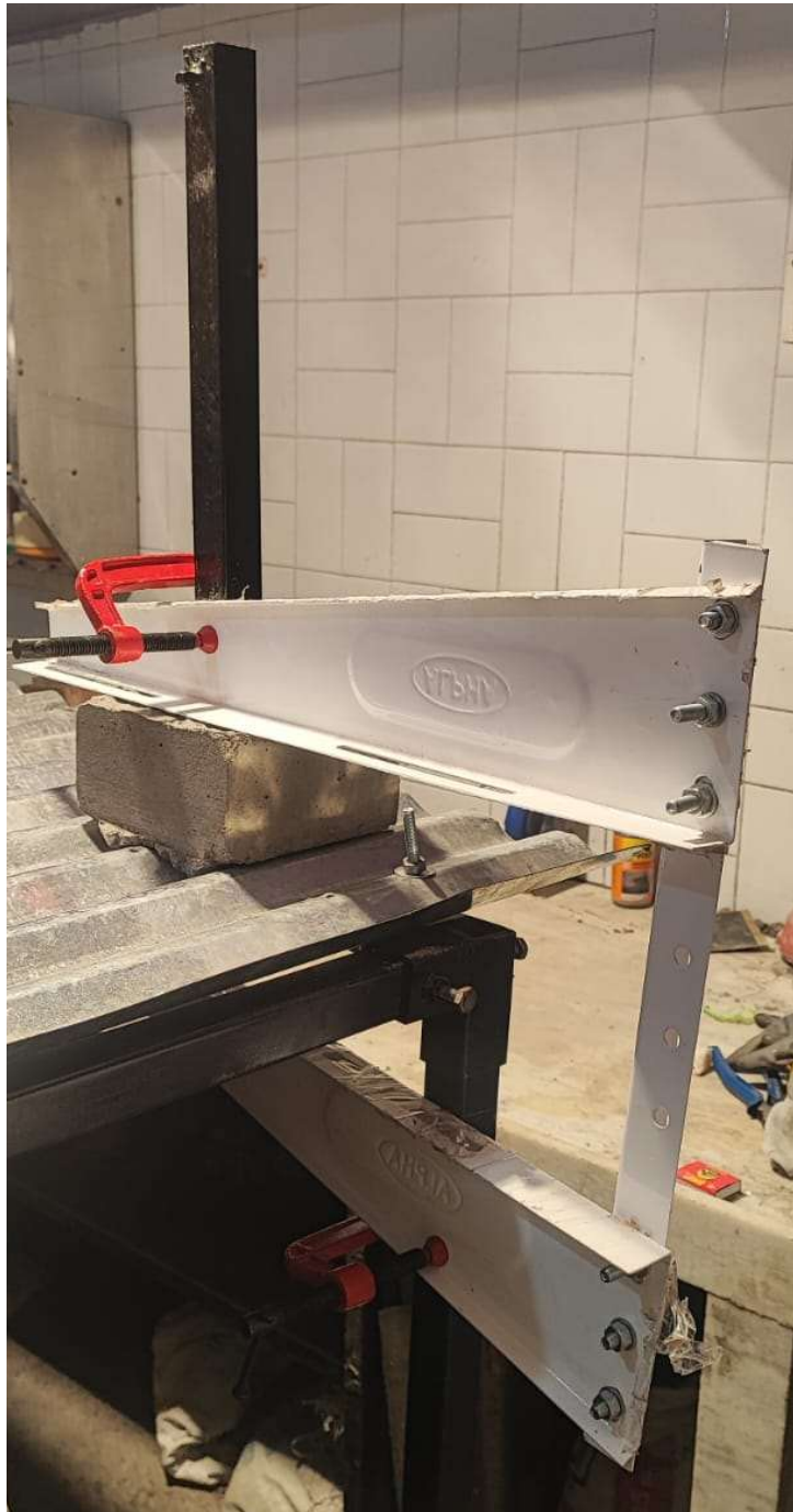
Fig 35.2.1-2 : Prototyping the Clamp-Based Support for Space Frame
