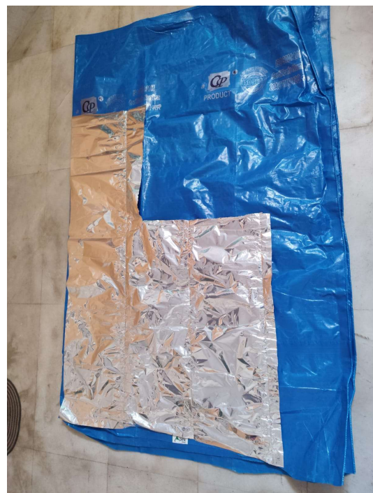
Fig 37.10.2-3 : MLP Sheet Placed Over Tarpaulin for Alignment and Size Verification
