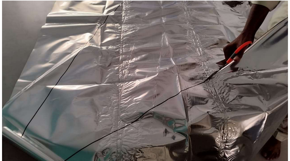
Fig 37.9.2.1.4-1 : Cutting of MLP according to measurements taken
