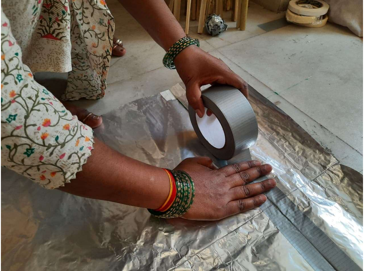
Fig 37.1.2-12 : Placing paper tape for marking 3 inch loop
