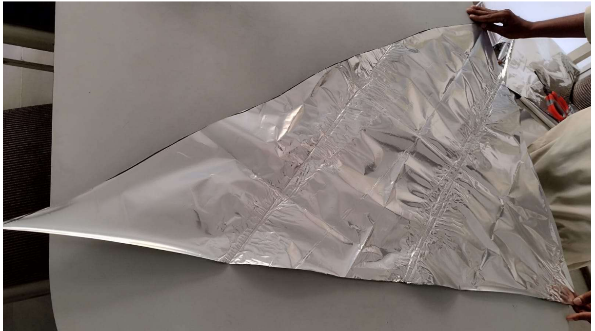
Fig 35.8.1-1 : Cutting of MLP Sheets into Triangular Shapes
