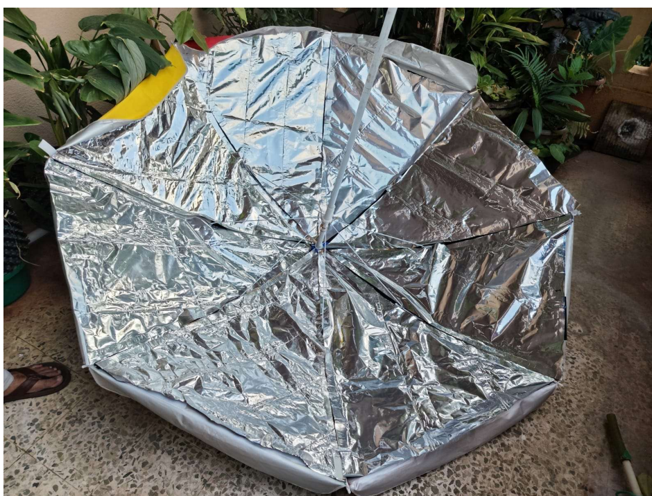
Fig 37.9.2.1.6-1: Shiny (reflective) side of MLP panels facing upward full umbrella covered, visible from top, showing the silver reflective surface of MLP across all 8 segments
