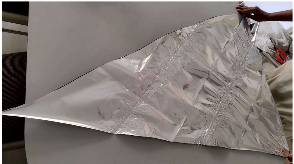
Fig 37.9.2.1.4-2 : MLP cut in Triangular shapes
