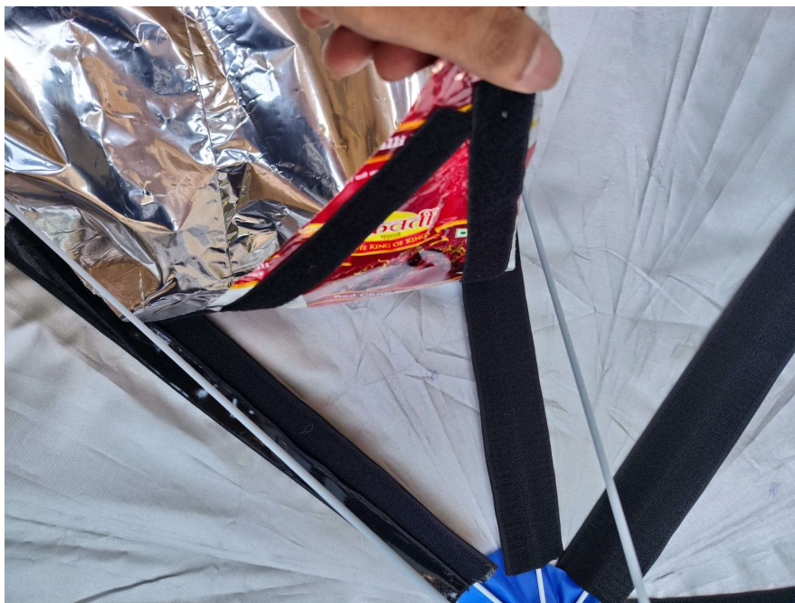
Fig 37.9.2.1.5-1 : MLP triangle is attached to umbrella with loop side(soft velcro) Attached to mlp non shiny side
