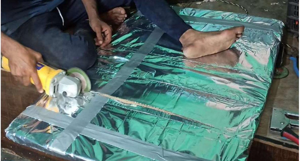
Fig 37.2.5-5 : Cut the whole panel
