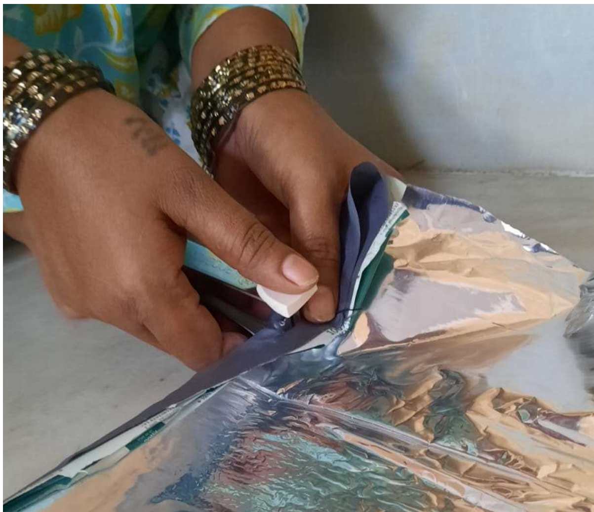
Fig 37.1.2-17 : Stapling the edge along the length.
