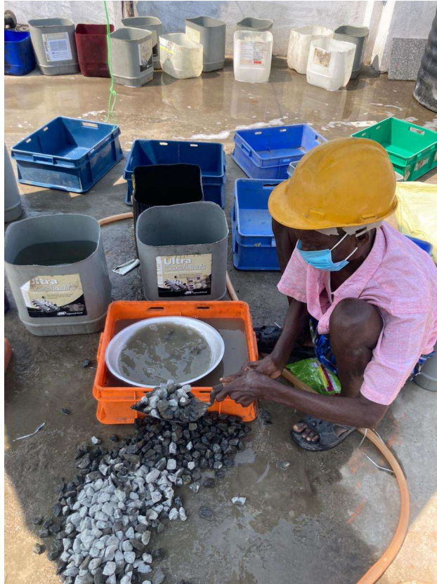
Fig 37.4.2-6 : Washing concrete chips
