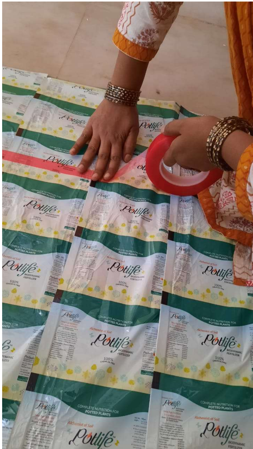
Fig 37.1.2-15 : Attaching high strength double side sticky tape for sticking 3 MLP layers
